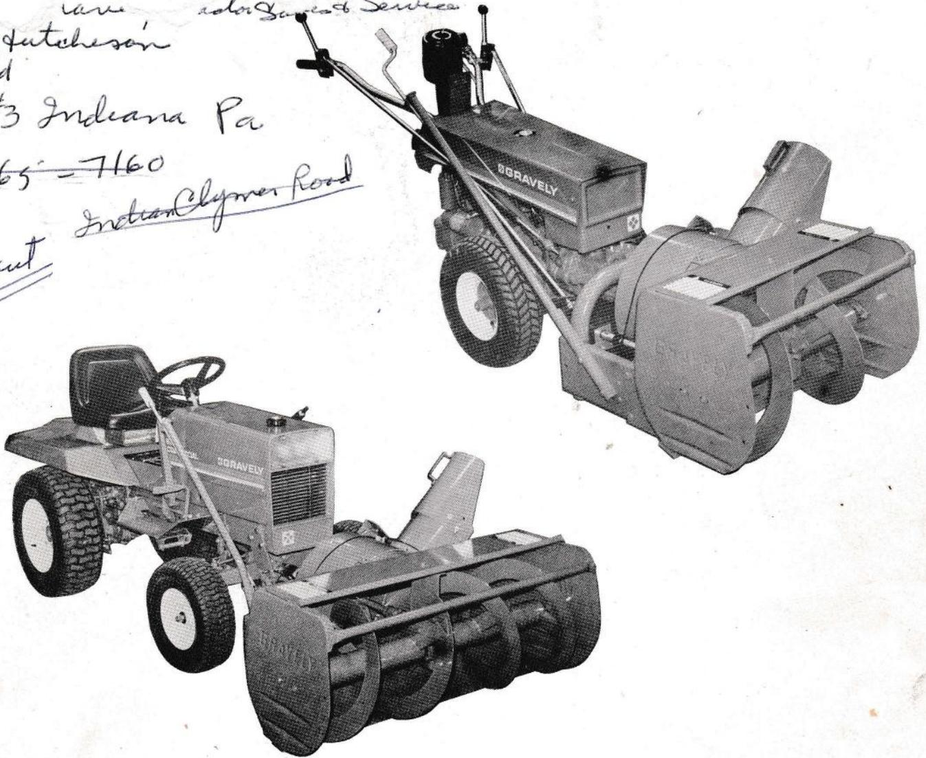
The 28 Inch and 34 Inch Snowblowers are used with Gravelly two wheel tractors. The 38 Inch and 44 Inch Snowblowers are used with Gravelly four wheel tractors.
