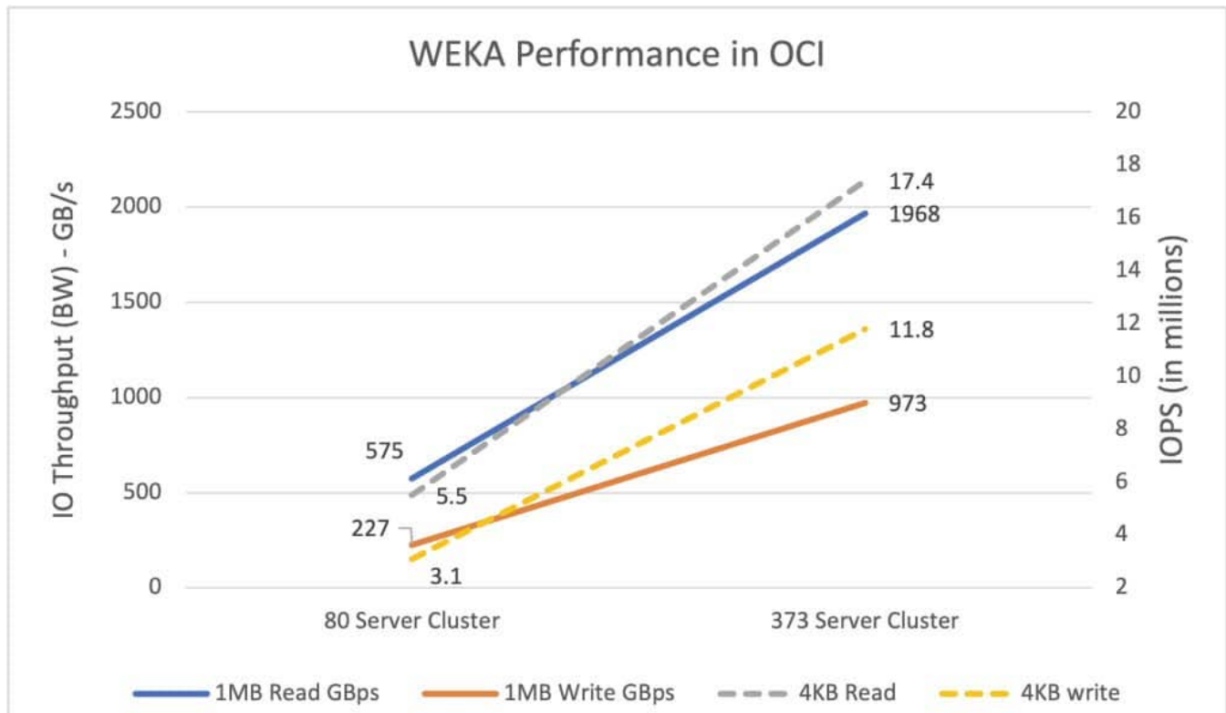
Figure 21: Performance at scale using WEKA in Oracle Cloud Infrastructure
