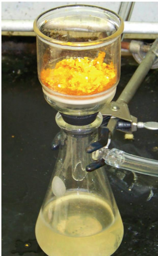
**Figure 4.16** Precipitate may be removed from a reaction mixture by filtration.
