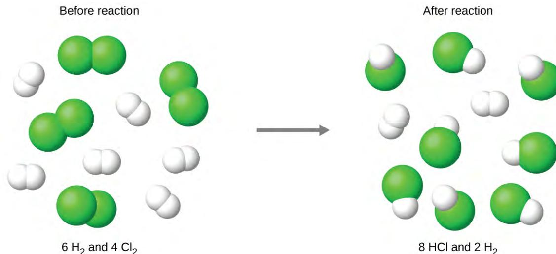
**Figure 4.13** When H<sub>2</sub> and Cl<sub>2</sub> are combined in nonstoichiometric amounts, one of these reactants will limit the amount of HCl that can be produced. This illustration shows a reaction in which hydrogen is present in excess and chlorine is the limiting reactant.
