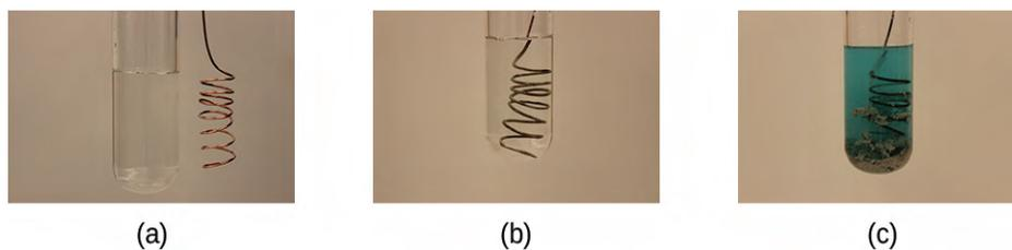
**Figure 4.8** (a) A copper wire is shown next to a solution containing silver(I) ions. (b) Displacement of dissolved silver ions by copper ions results in (c) accumulation of gray-colored silver metal on the wire and development of a blue color in the solution, due to dissolved copper ions. (credit: modification of work by Mark Ott)
